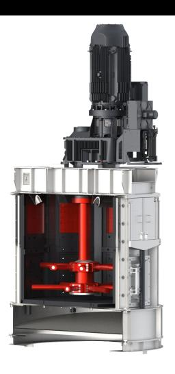
Stirred media detritor (SMD) is a fluidized, vertical stirred mill designed for optimum grinding efficiency for fine and ultrafine grinding products. SMDs have the capacity to operate continuously at full load power draw with no steel contamination of the product. They are suitable for both open and closed-circuit operation.
